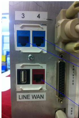
LAN Ports Local Area Network These Ports are for the connection from your PC to the MLogger
