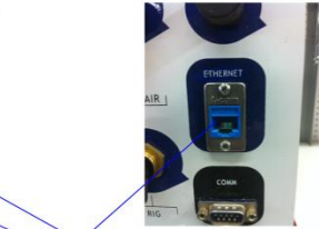
LAN Ports Local Area Network These Ports are for the connection from your PC to the MLogger
